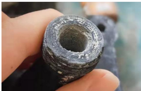
图 8 因堵塞导致报废的喷头 Fig.8 Printheads scrapped due to clogging
