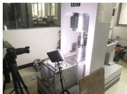
图 15 RMT-150C 岩石力学试验设备 Fig.15 RMT-150C rock mechanics test equipment
